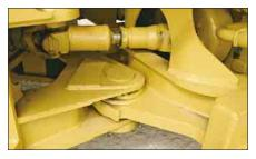
**Spread Hitch.** The distance between the upper and lower hitch plates is important for machine performance and component life. The Cat spread hitch design provides excellent load distribution and bearing life. Both the upper and lower hitch pins pivot on double tapered roller bearings – improving durability by distributing both vertical and horizontal loads over a larger surface area. The wide opening also provides excellent service access.
