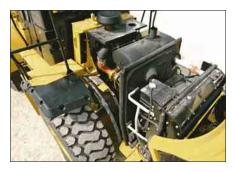
A single mechanical lift cylinder with manual back-up opens the hood. The tilting hood provides excellent access to the engine compartment, and if necessary, the entire hood can be removed with the built-in lift points. With the hood closed, quick checks of engine oil level and the coolant sight gauge can be completed through the side service doors.
