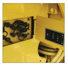
**Remote Pressure Taps.** Pressure taps for the steering and hydraulic systems, transmission (optional) and brakes are grouped behind an access panel just below the right-side service platform.
